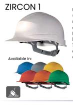
UV-resistant high density polyethylene (HDPE) or polypropylene (PP) safety helmet. Low density (LDPE) polyethylene cradle with 8 fixing points. Sweat band. Manual adjustment: head sizes 53/63 cm Electrical Insulation up to 1000 V.A.C. or 1500 V.D.C. Standard holes for accessories. Anchorage for chin straps with 2 or 4 points.
