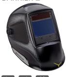
Helmet for electric arc welding with self-obscuring screen. Can be used for MIG, MAG, TIG and plasma welding requiring 9 to 13 shade protection. Can be used in shade 5 to 9 for low intensity or flame welding. Can be used for grinding in shade 4.
