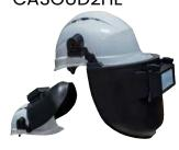
Polypropylene welding face shield, to be used on safety helmets. For all types of welding that requires shade 11 protection. Sold ready to use: fixed screen equipped with one clear poly-carbonate filter (FILTER-IN), flip-up screen equipped with one shade 11 filter (FILTER-11), protected by one clear polycarbonate filter (FILTER-IN). Dimensions of the filters: 108 x 51 mm.
