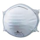
Box of 10 active charcoal non woven synthetic fibre disposable masks FFP2 for organic vapours (for concentration < VME). Protection against harmful odours (welding fumes for example). Moulded mask. Nose clip for adjustment. Foam edge under nose clip. High performance exhalation valve. DOLOMIA optional test for longer continuous wear time.
